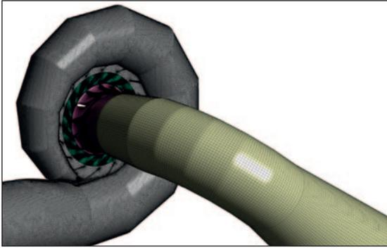
Fig. 3. Visualization of the meshes, distributor and runner.
