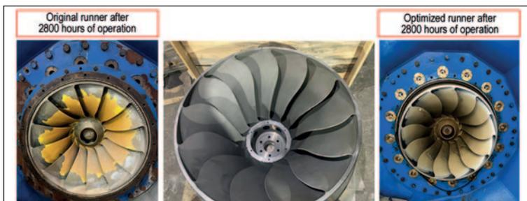
For Reference Project No. 2, Fig. 11 shows the original runner (left) and the optimized design (right). Both pictures refer to an operation time of around 2800 hours. The operational experience clearly proves the improved resistance to erosion.
