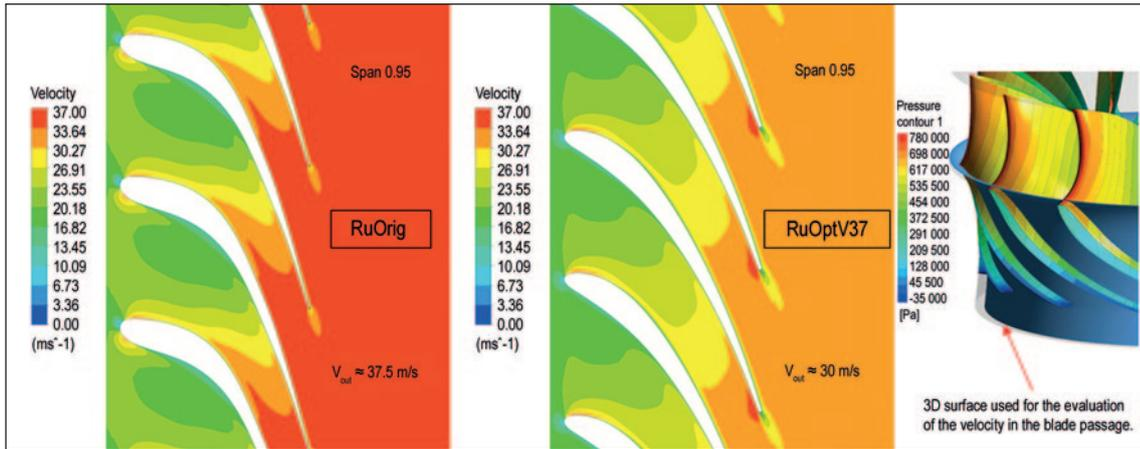
Fig. 8. Blade-to-blade view of the velocity in the blade passage at 95 per cent blade height at  $Q \approx 10 \text{ m}^3/\text{s}$  and  $H = 108 \text{ m}$  (left view, original runner; and, middle view: optimized runner).
