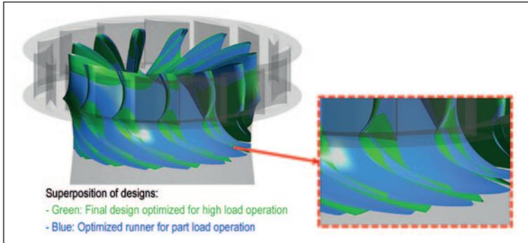
Fig. 10. Superposition of the runner optimized for high load conditions and the one specifically designed for deep part-load operation.
