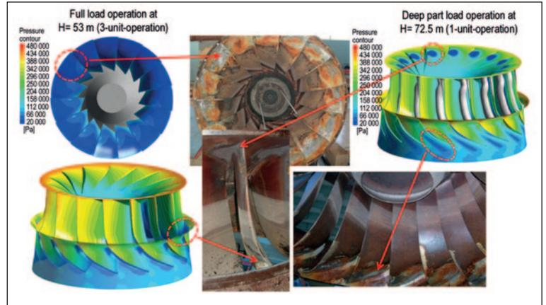
Fig. 4. Comparison of low-pressure zones calculated using CFD, and damage found on the original runner.
