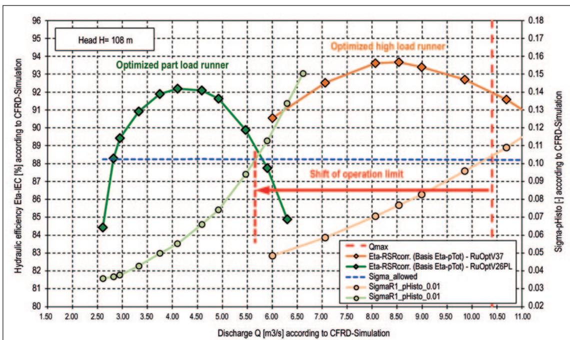
Fig 9. Comparison of efficiency and cavitation characteristics of the optimized high-load and low-load runner.
